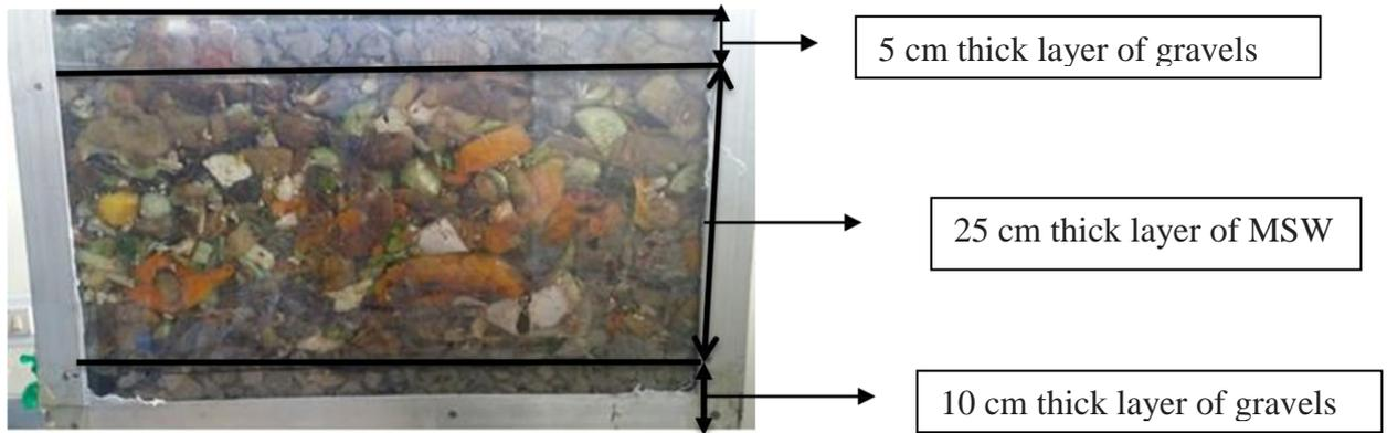
**Figure 3.4** Complete filling of reactor
