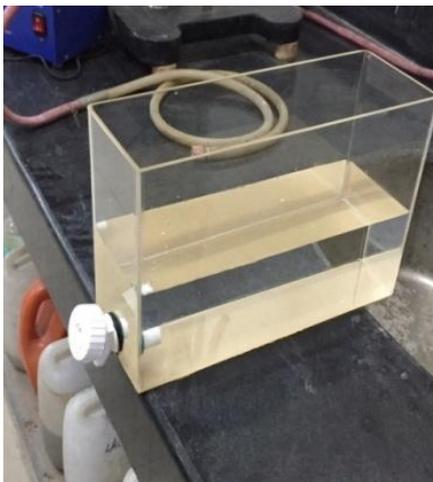
**Figure 3.7** Aeration tank filled with water
