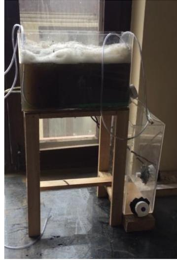
**Figure 3.6** Operation of lab scale ASP
