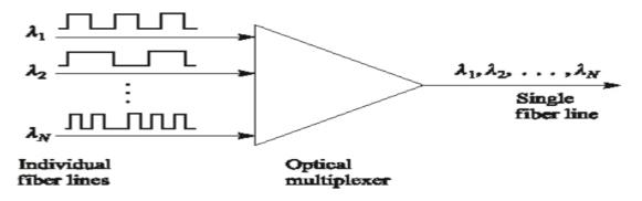
Figure 1.2 Wavelength Division Multiplexing [2]
