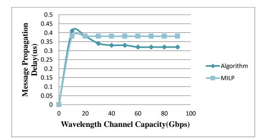
Figure 5.16 Message Propagation Delay VS Wavelength Channel Capacity for 11 Node Network
