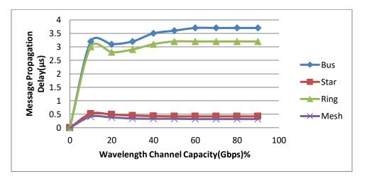
Figure 5.5 Message Propagation Delay (µs) VS Wavelength Channel Capacity (%Gbps) for 11 Node Network
