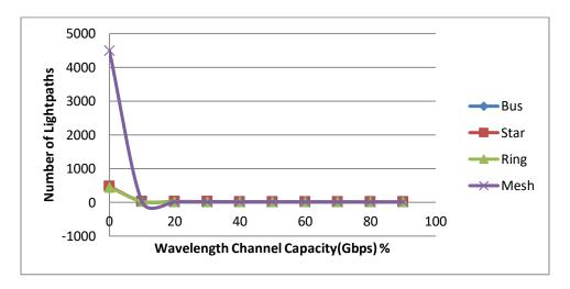
Figure 5.3 Number of Lightpaths VS Wavelength Channel Capacity (%Gbps) for 11 Node Network
