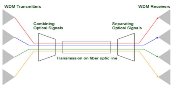
Figure 1.3 Wavelength Division Multiplexing Working Principle[2]
