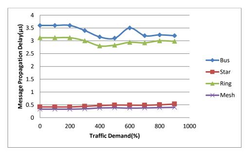
Figure 5.11 Message Propagation Delay ( $\mu$ s) VS Traffic Demand (%) for 11 Node Network
