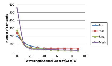
Figure 5.2 Number of Lightpaths VS Wavelength Channel Capacity (%Gbps) for 5 Node Network
