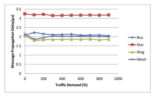
Figure 5.10Message Propagation Delay ( µs)VS Traffic Demand (%) for 5 Node Network
