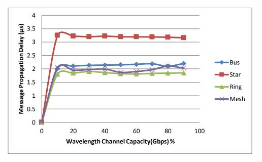
Figure 5.4Message Propagation Delay(µs)VS Wavelength Channel Capacity (%Gbps) for 5 Node Network
