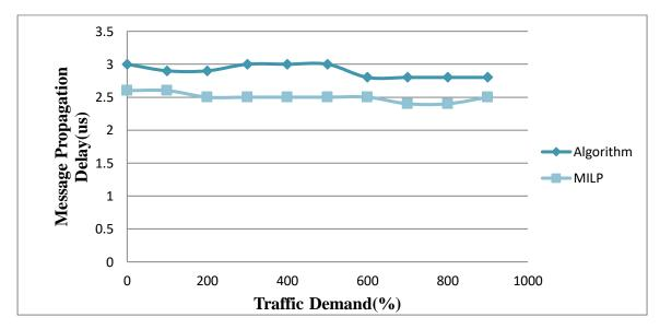
Figure 5.13 Traffic Demand VS Message Propagation Delay(us) for 11 Node Network
