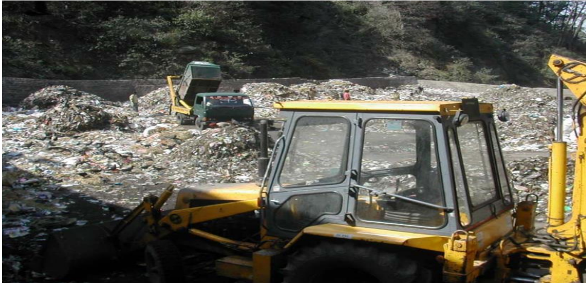
Figure 3.9 Turning of waste using JCB at Darni Ka Baghichha.
