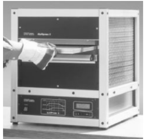
Fig. 11.5 Typical lamination press for multi-layer boards (Muller, 2000)
