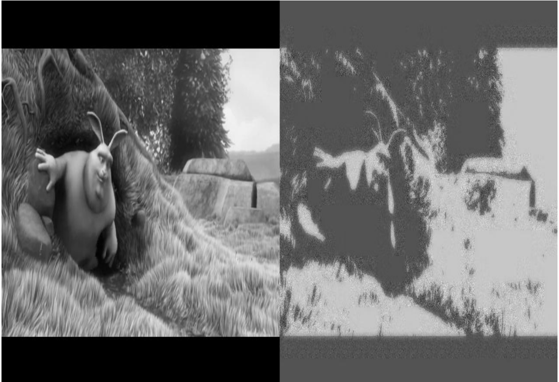
Figure 5.6(b): Simulation result for 22 th frame when CS applied is on video
