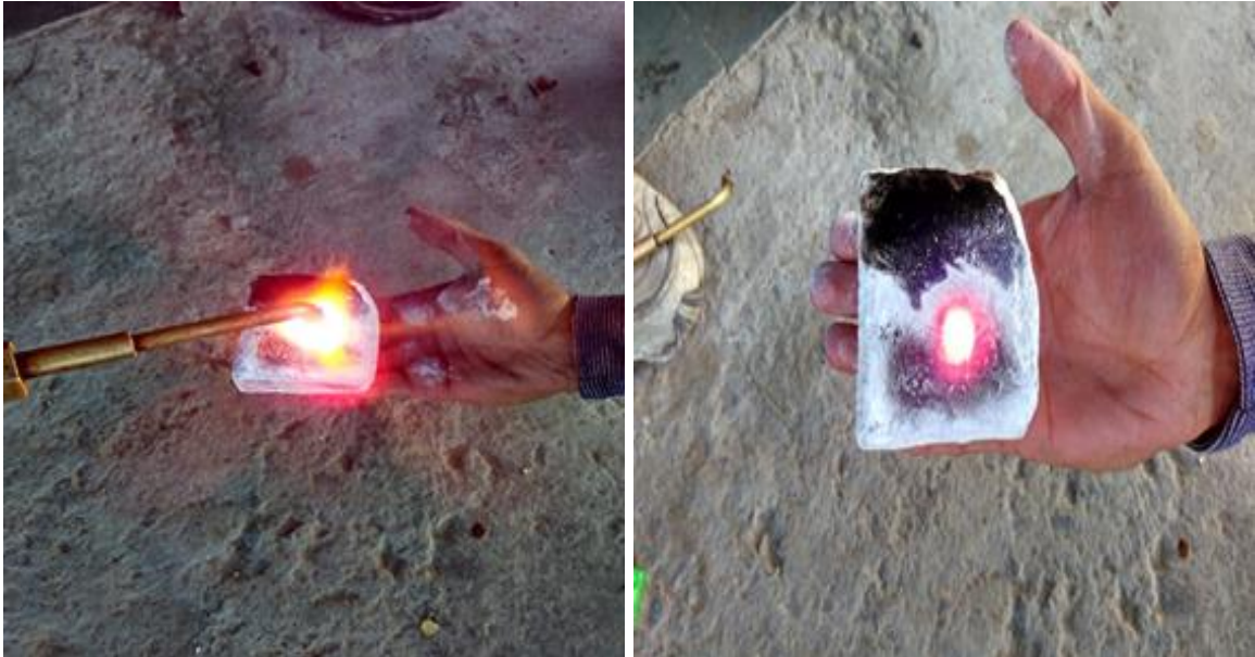
Figure 4.7 – MOC sample exposed to flame
