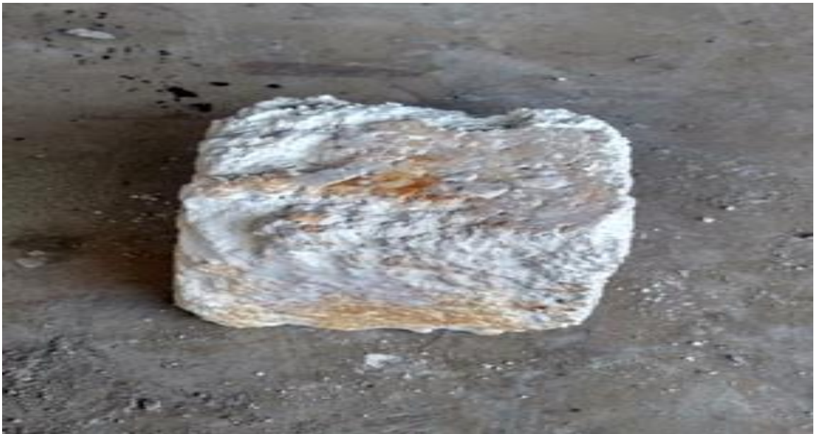
Figure 4.5 – Deterioration of the MOC cube when exposed to water
