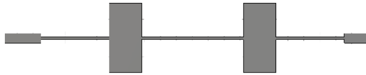
Figure 4.3: Fifth Order Stepped Impedance LPF
