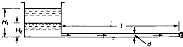
Fig. 13-6. Time of emptying a tank.
