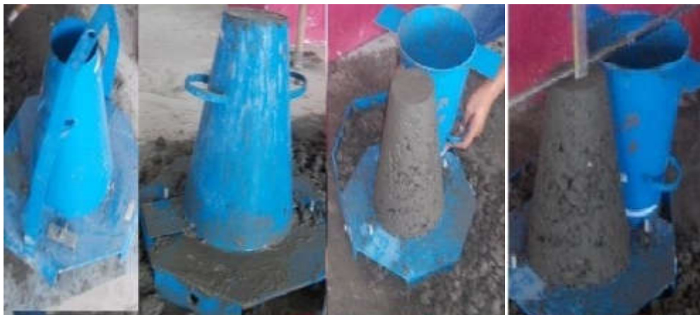
Figure (4.1) Slump value determination
