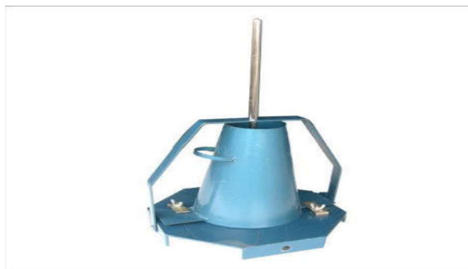
Figure (3.5) Slump cone
