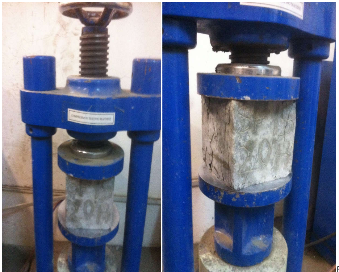
Figure (3.6) Testing of cubes
