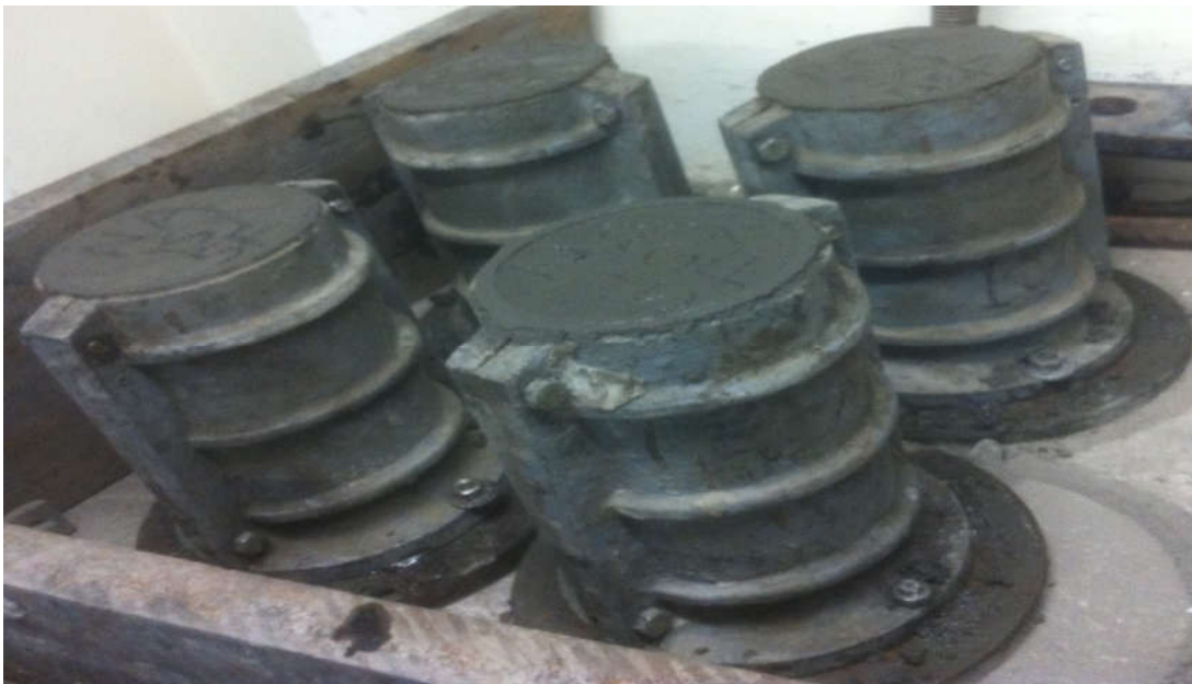
Figure (3.4) casting of cylinder
