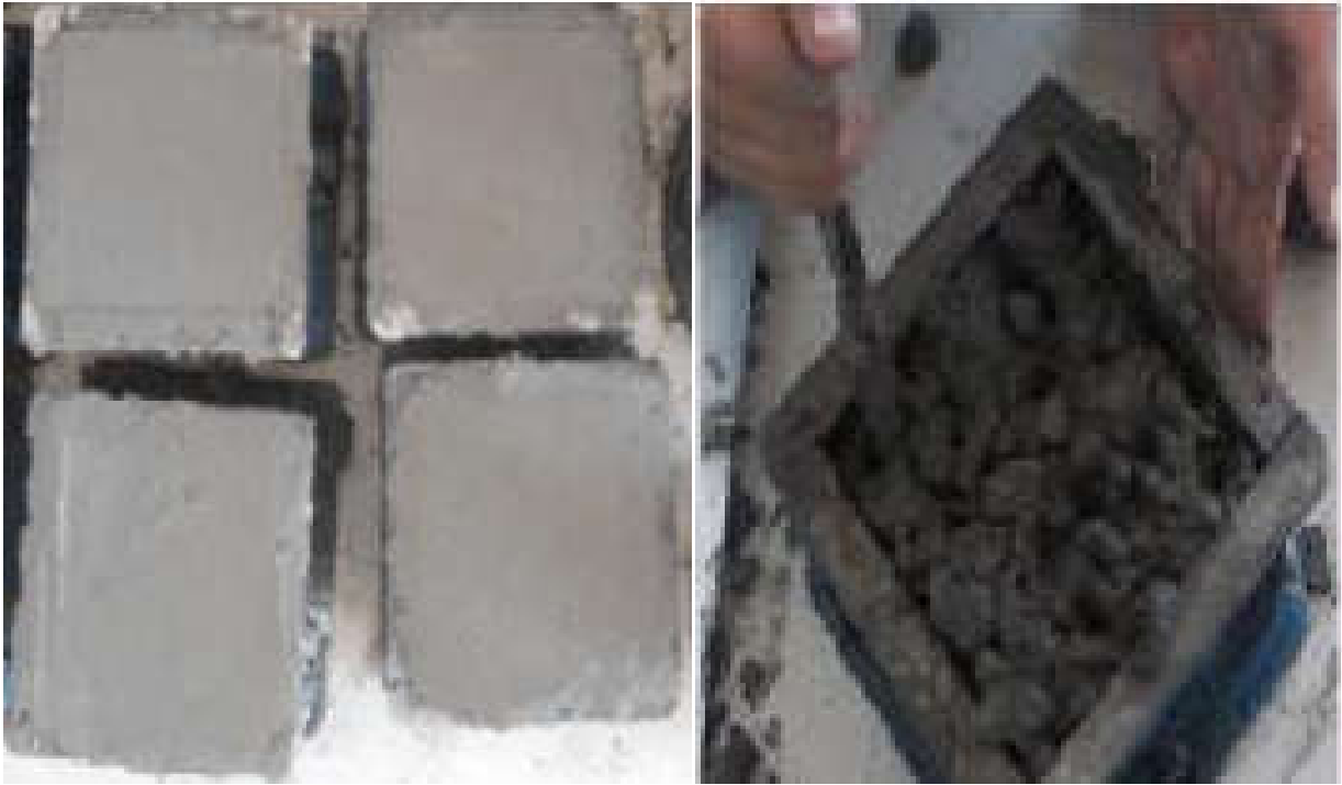
Figure (3.3) Casting of cubes
