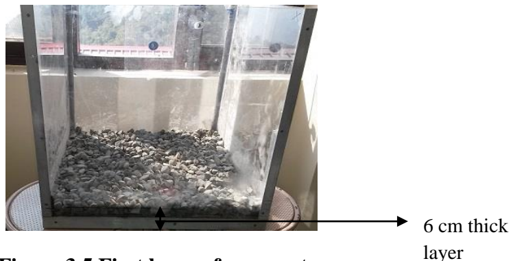
Figure 3.5 First layer of aggregates
