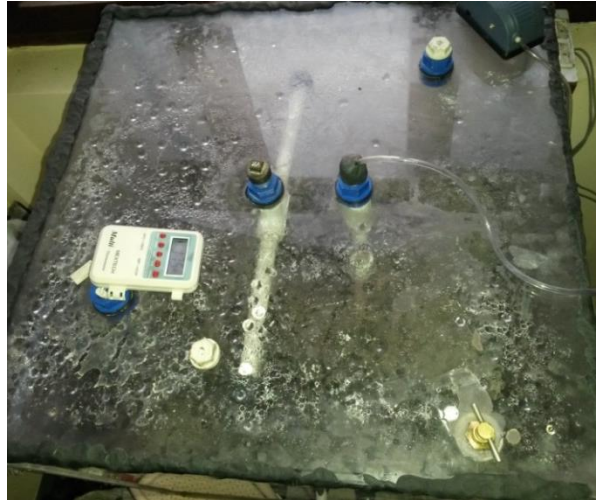
Figure 3.5.3 Water droplets on the wall of reactor
