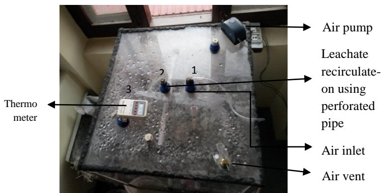
Figure 3.1 Top view of reactor
