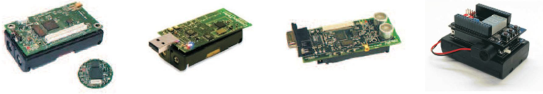
Figure 1.1: Typical sensor motes: MicaZ mote, Telos mote, Cricket mote and MITmot mote.
