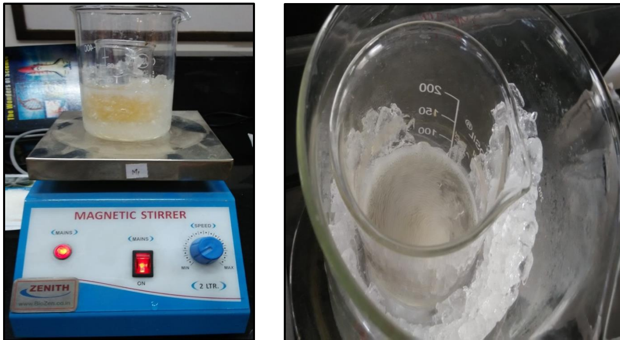
Figure 3: Setup for Ammonium sulphate precipitation
