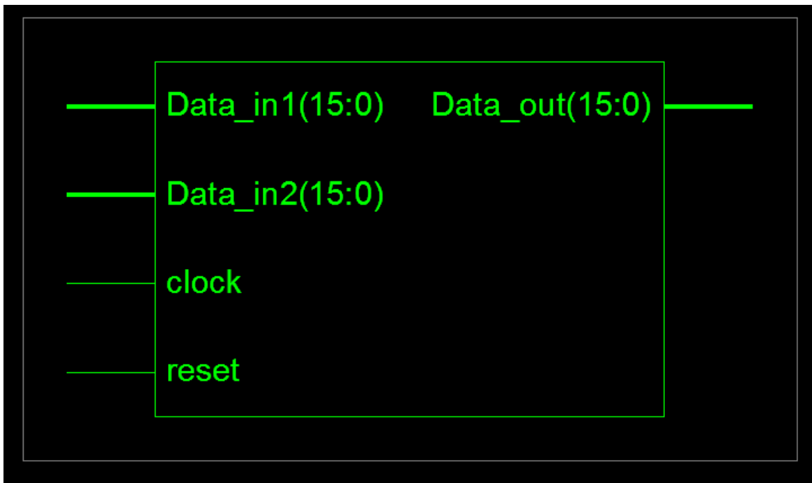
Fig. 4.1 Block Diagram of Convolution Unit
