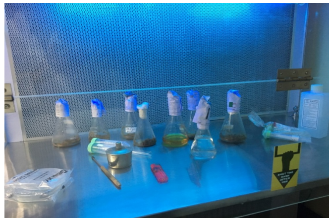
Figure 3.8: Use of UV to kill all the microbes
