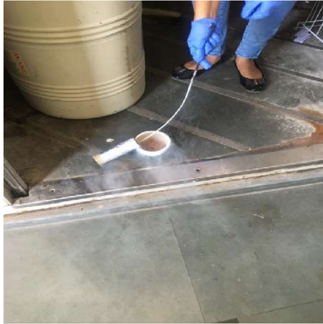
Figure 3.5: Using liquid nitrogen to crush the dried pomace
