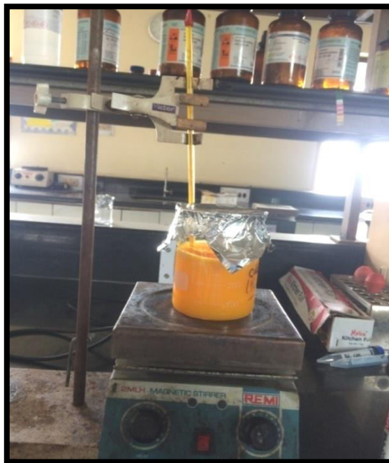
Figure 2.4: Experimental set up of Synthesis of CdS through solution growth method
