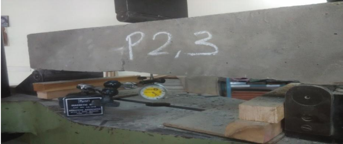
Figure 5.1: Experimental set-up for 3-point-bend test.
