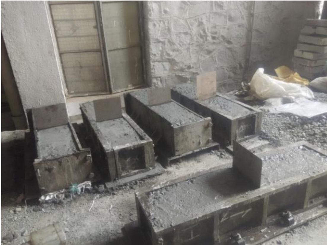
Figure 5.2: Casting and development of artificial notch using ply-wood.
