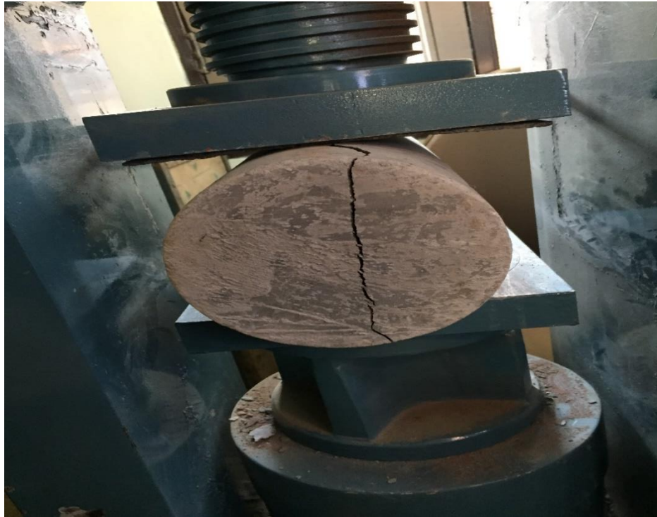
Fig. 4.3 Split Tensile Test
