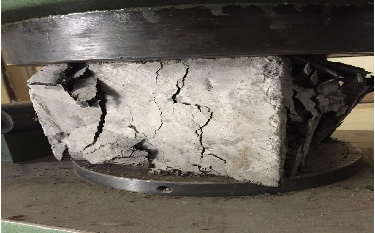
Fig.3.2:Cracking in FRC
