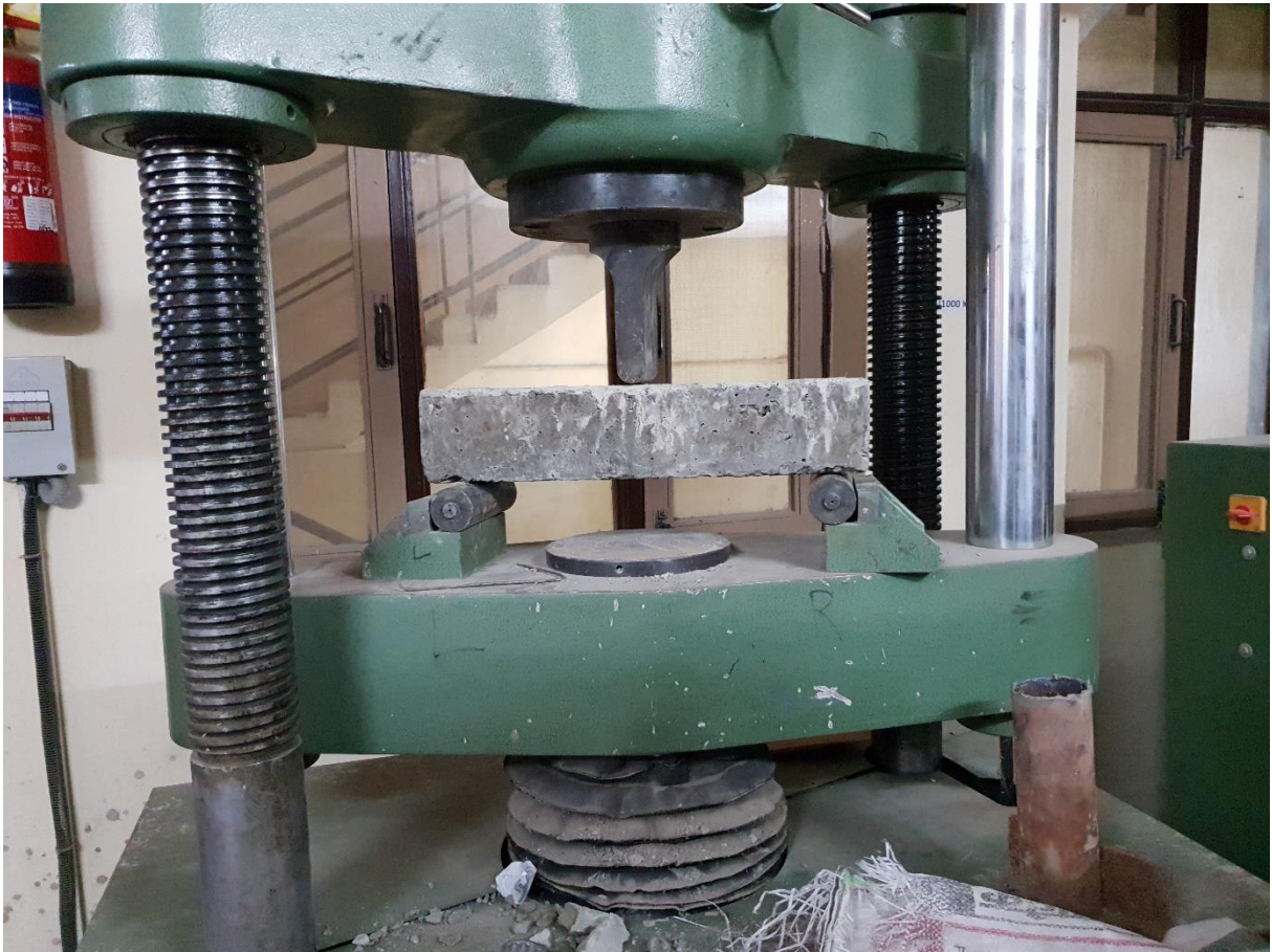
Fig 5.3 testing of beam under UTM (flexure)
