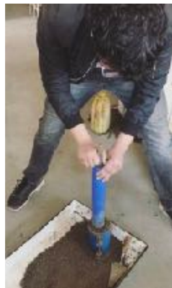
Fig 7.13 Proctor test in progress
