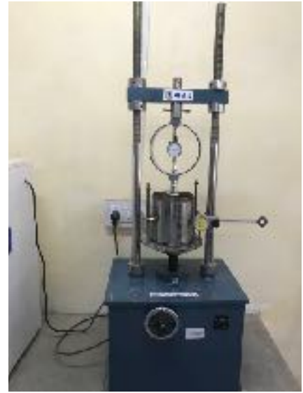
Fig 7.15 CBR test in progress.
