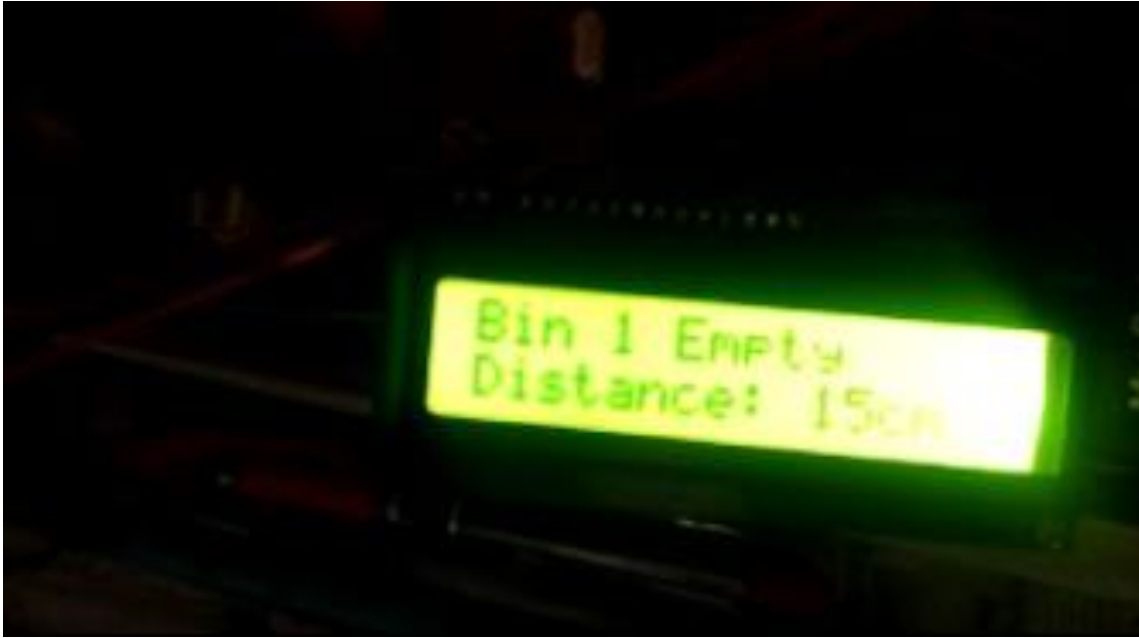
Figure 5.4: LCD Display showing Bin status and depth of the bin
