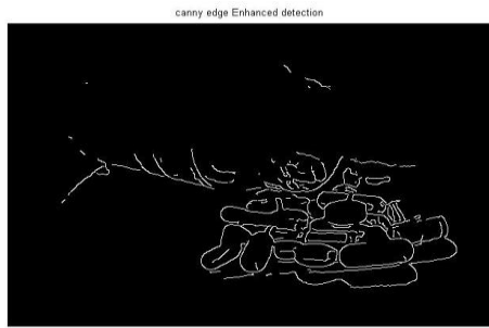
Figure 30(q): edge detected image after Applying homomorphic filter
