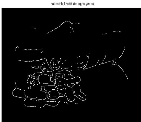
Figure 30(m): Edge detected image after applying combination of mode and median filter
