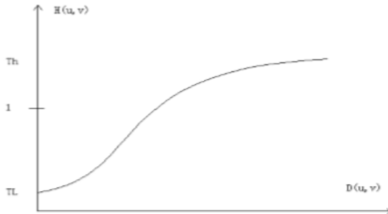
Figure 4: The Schematic Profile of Homomorphic Filter's Transfer Function H(u, v) [3]
