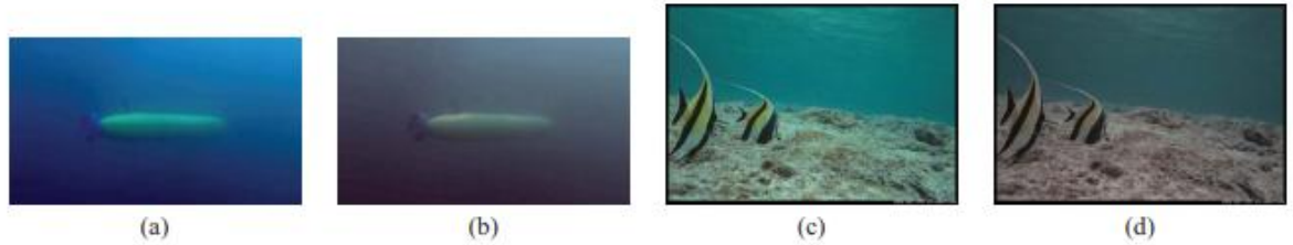
Figure 8: Image correction using quaternion method(a, c) Original image (b,d) Enhanced image [7]
