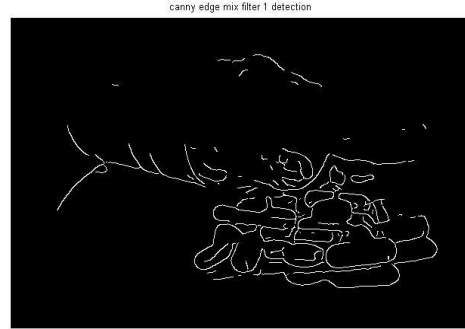
Figure 30(h): Edge detected image after applying combination of mode and median filter
