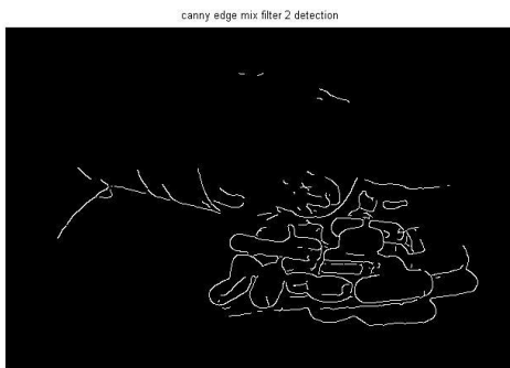
Figure 30(i): Edge detected image after Applying combination of mode and Bilateral filter
