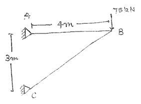
Q.5. For the given beam find the support reactions and slope at B by using Stiffness Matrix Method.
