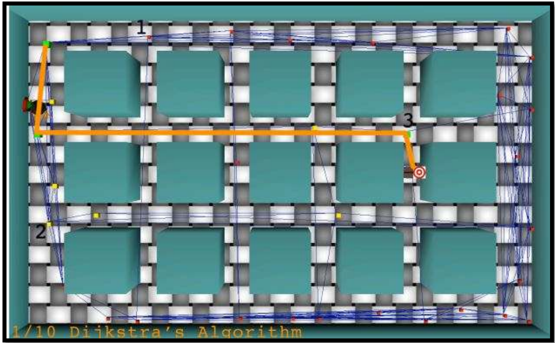
Figure 51. Testing Tool in Simulation 1, Dijkstra's algorithm
