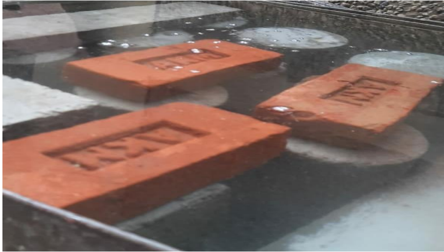
Fig 30. Curing red bricks
