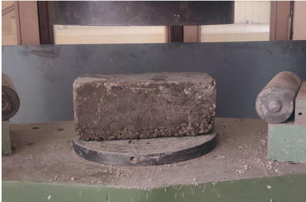
Fig 36. M7.5 specimen before testing on 7th day
