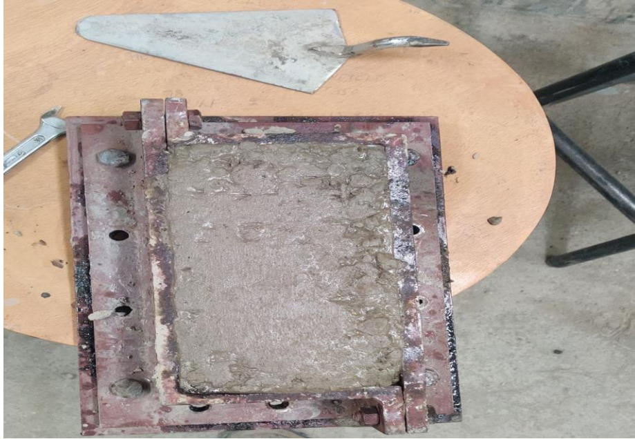
Fig 22. Properly casted mortar in moulds
