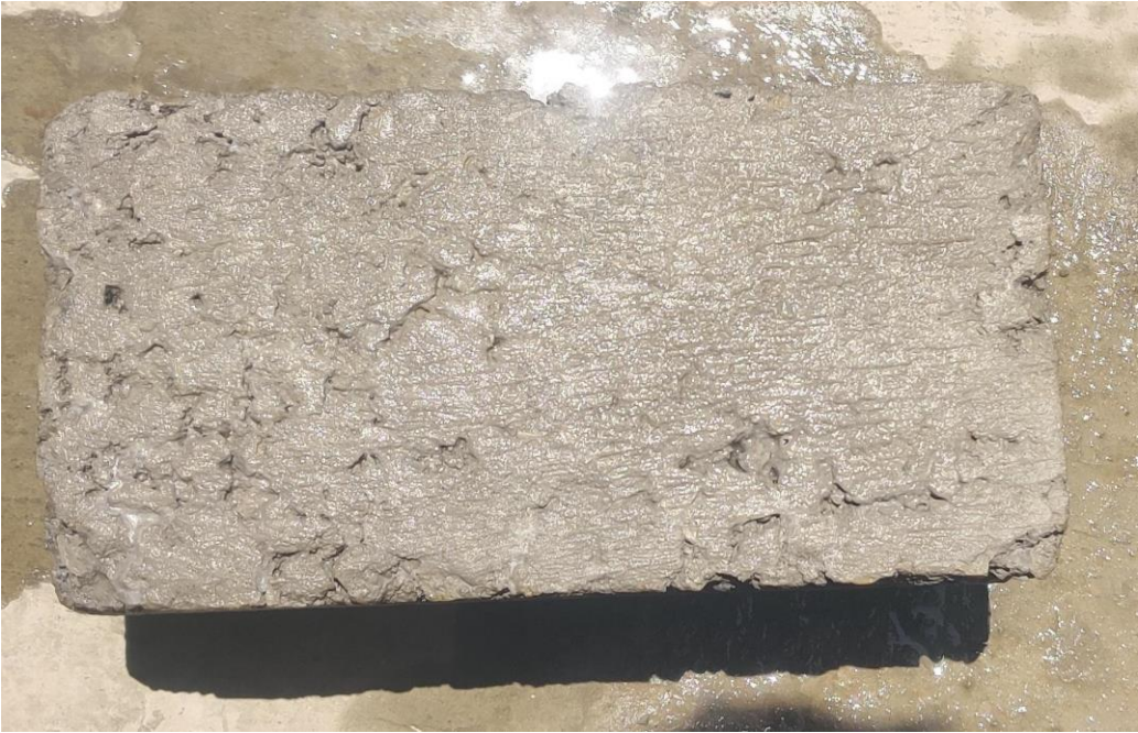
Fig 38. M7 specimen before testing on 14th day
