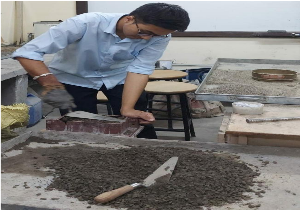
Fig 20. Putting mortar into the moulds
