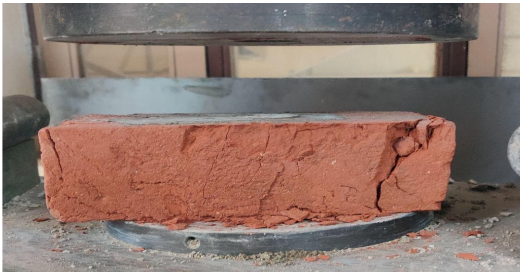
Fig 33. Red bricks after testing
