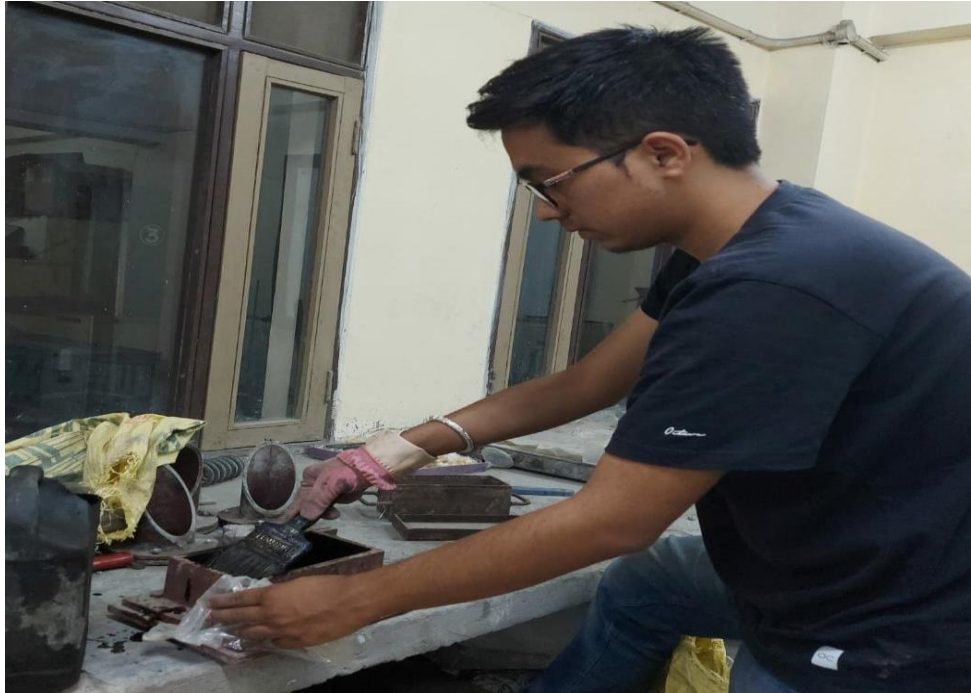
Fig 12. Applying oil to the moulds
