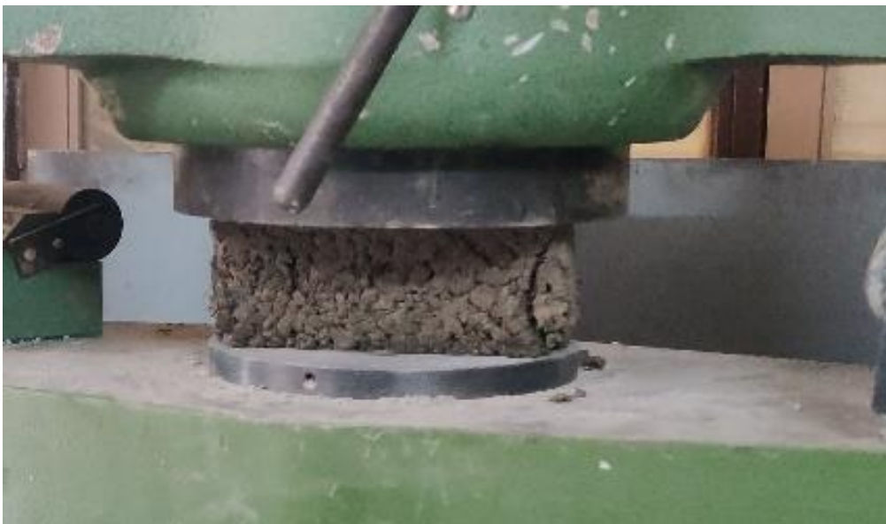
Fig 41. M10 brick in Universal testing machine on 7th day
