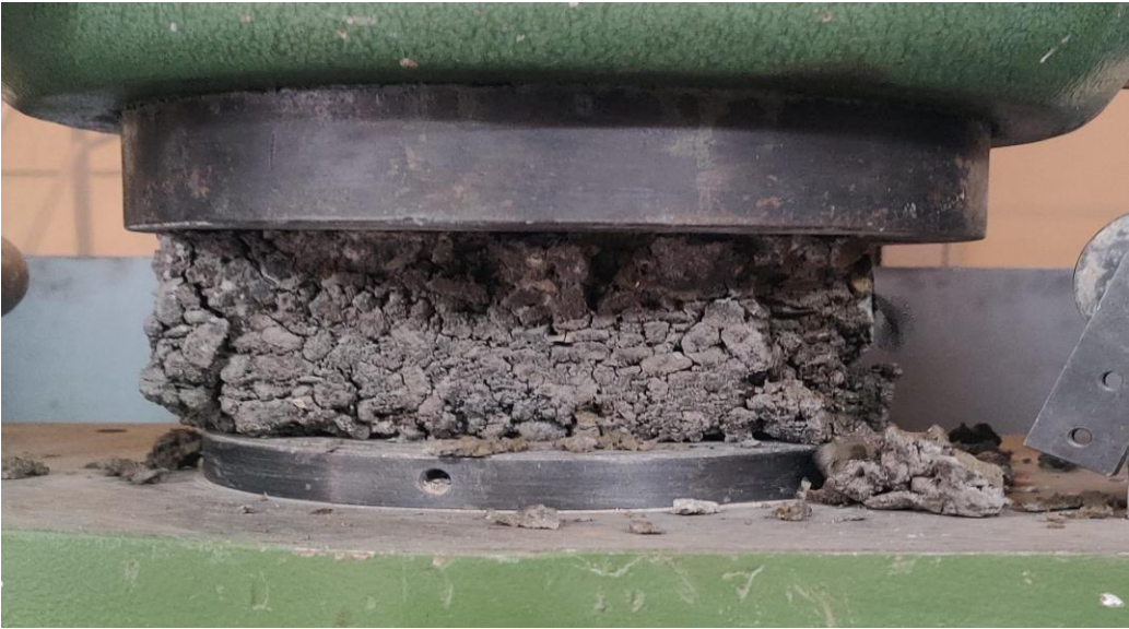
Fig 39. Performing compressive strength test on 14th day on M7.5 specimen
