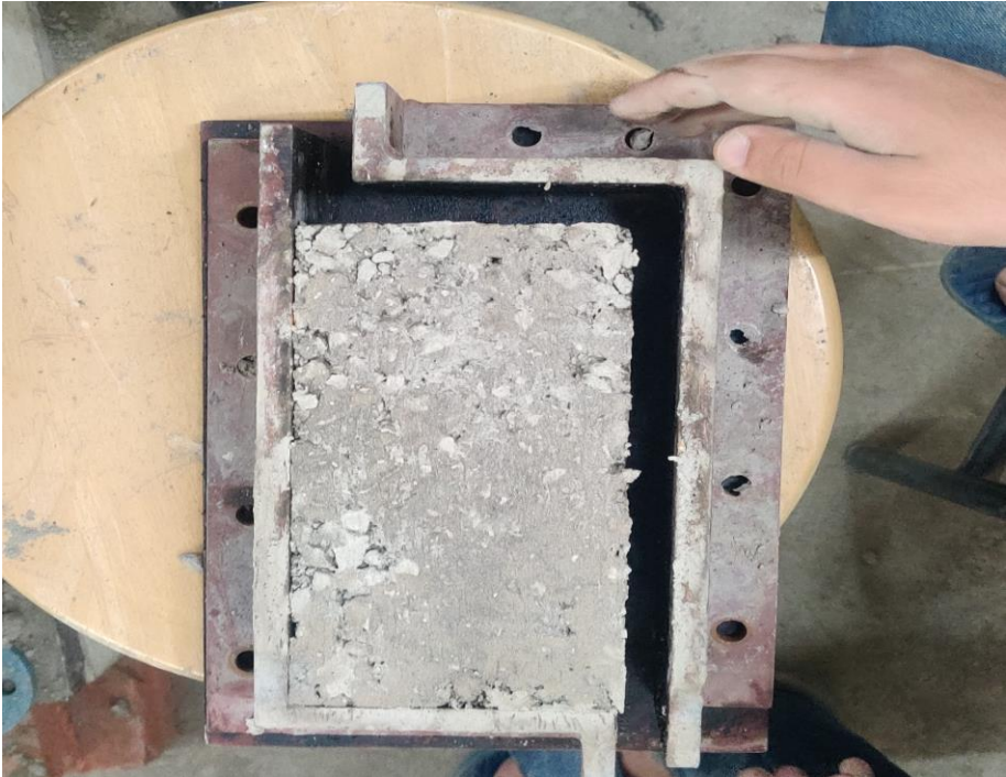
Fig 26. Removing sides carefully
