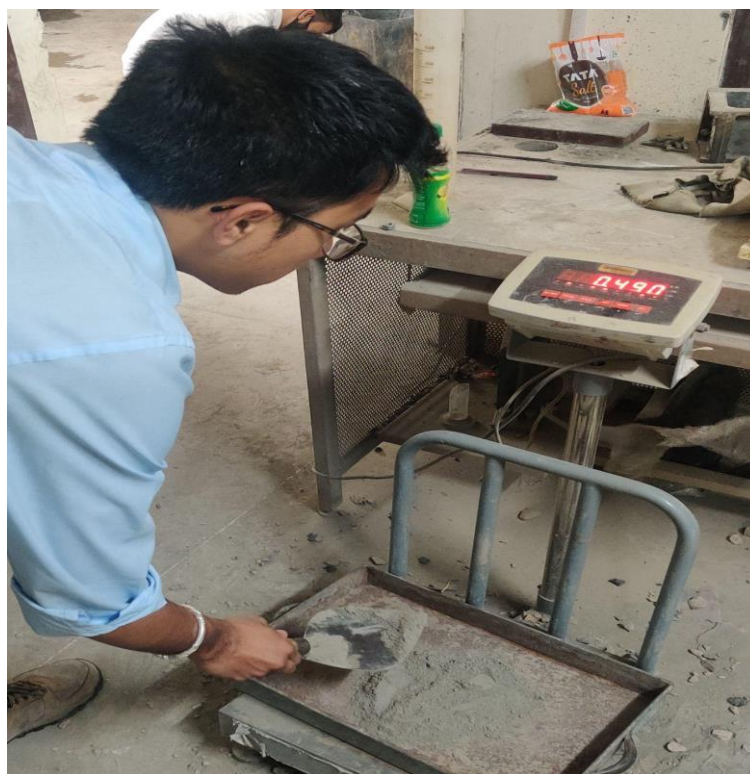
Fig 15. Weighing of cement
