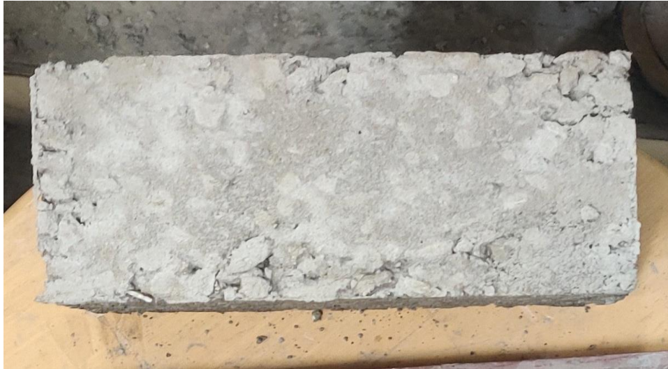
Fig 34. M5 specimen before testing
