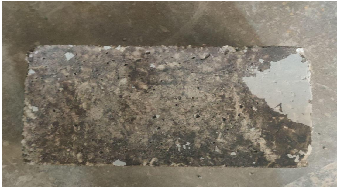
Fig 40. M10 specimen on the 7th day before testing
