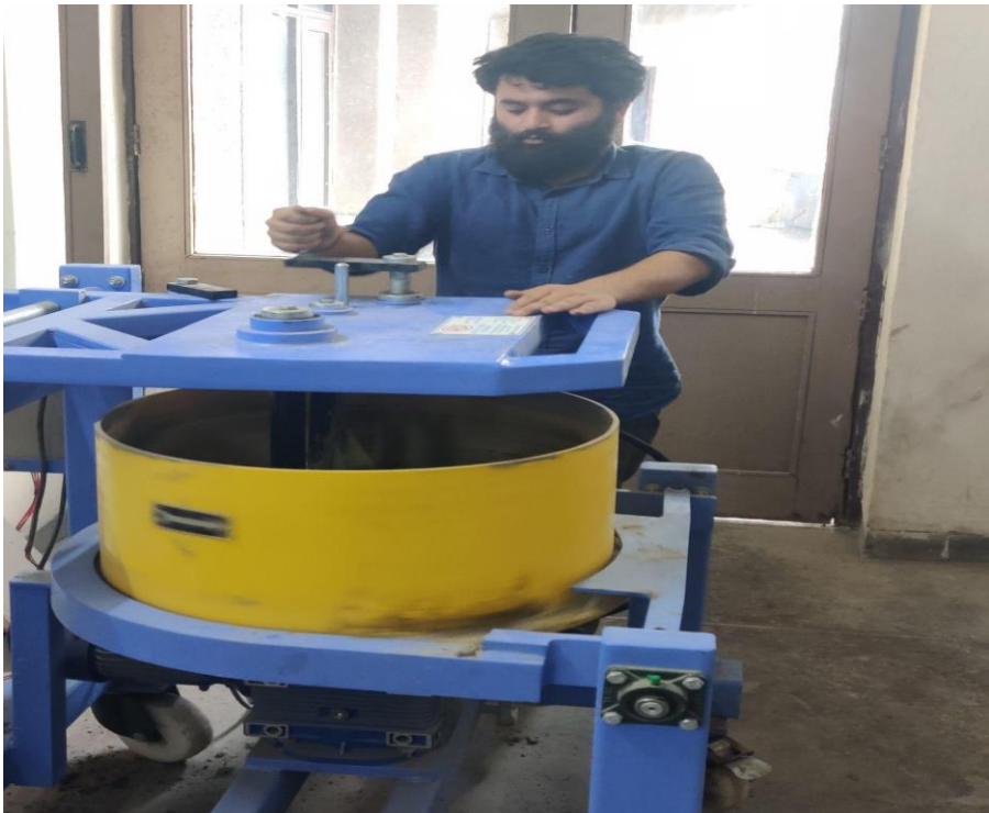
Fig 17. Mixing materials together in concrete mixer
