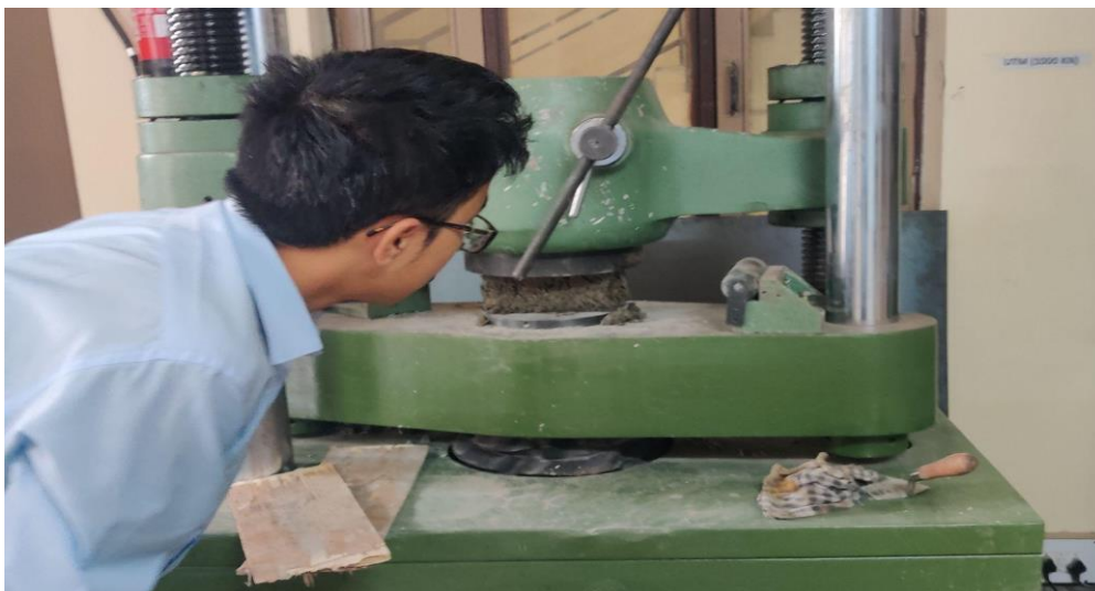
Fig 37. Performing compressive strength test at day 7 for M7.5 bricks
