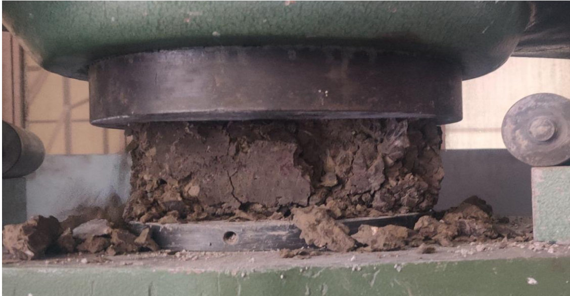
Fig 42. M10 specimen on 14th day in Universal testing machine
