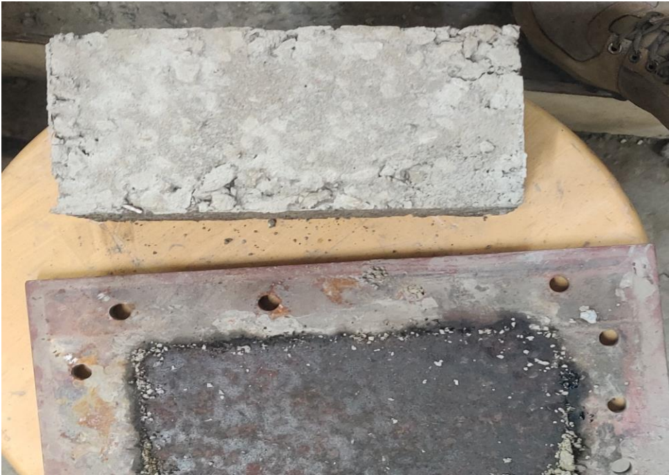
Fig 27. Demoulding of M7.5 mix grade concrete bricks
