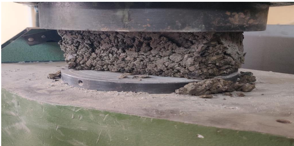
Fig 35. Compressive strength test on M5 bricks
