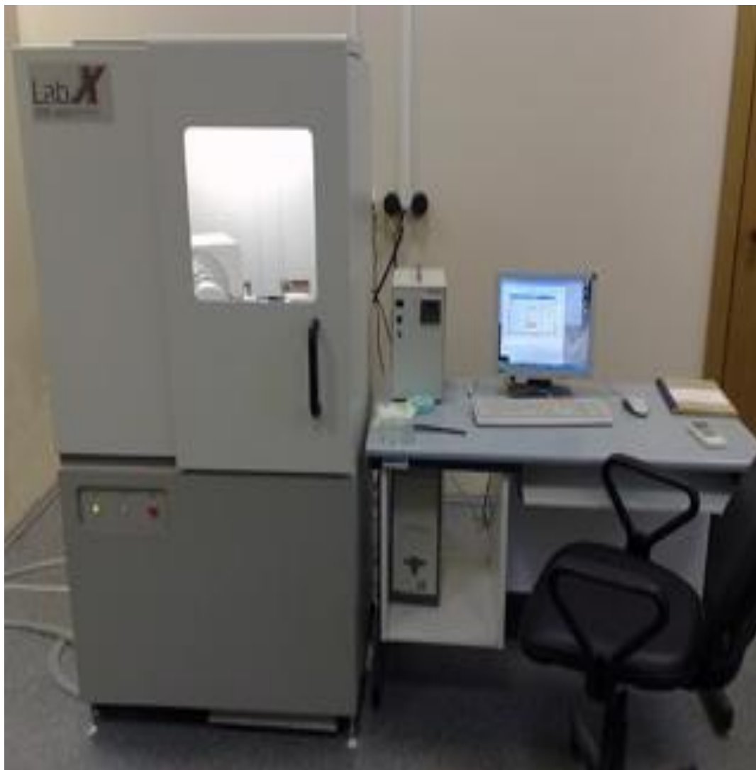
Figure 2.3: Shimadzu (XRD 6000) X-Ray diffractometer employed for XRD studies
