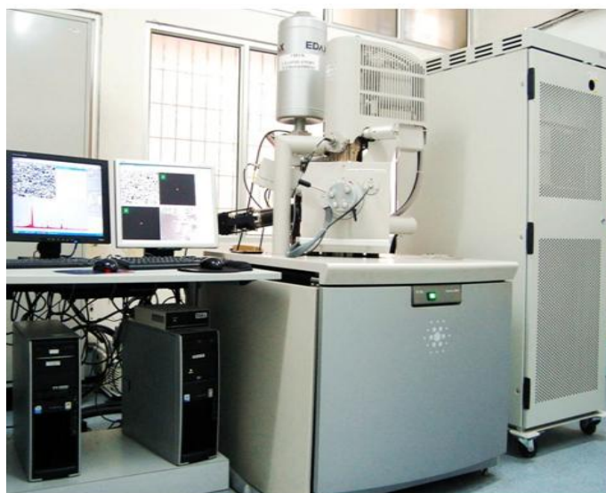
Figure 2.7: Quanta 200 FEG Field effect scanning electron microscope
