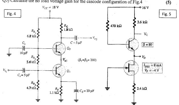
Q6) Determine  $V_D$  and  $V_C$  for the network of Fig. 5.
