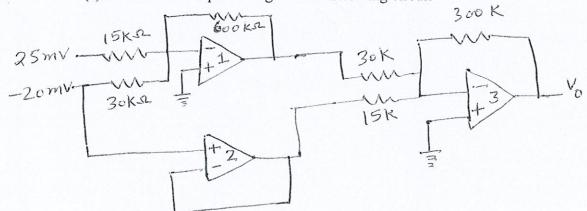
(b). Design an input offset voltage compensating network for the given circuit. Op-amp is IC  $\mu A715$  with  $v_{io} = 5 mV$  maximum and supply voltages are +15volt and -15volt. Draw the complete circuit diagram.
