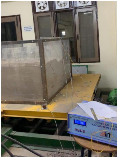
Fig. 3.14 (a) Shake table with whole setup
