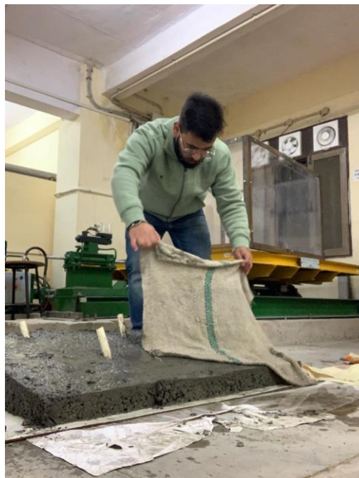
Fig.3.8 (d) Curing with the help of cloth and sack
