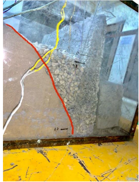
Fig. 3.15 Retaining Wall with Backfill failure
