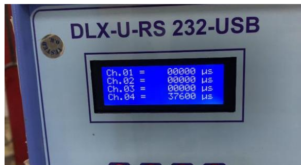
Fig.3.4 Data Logger to measure strain values
