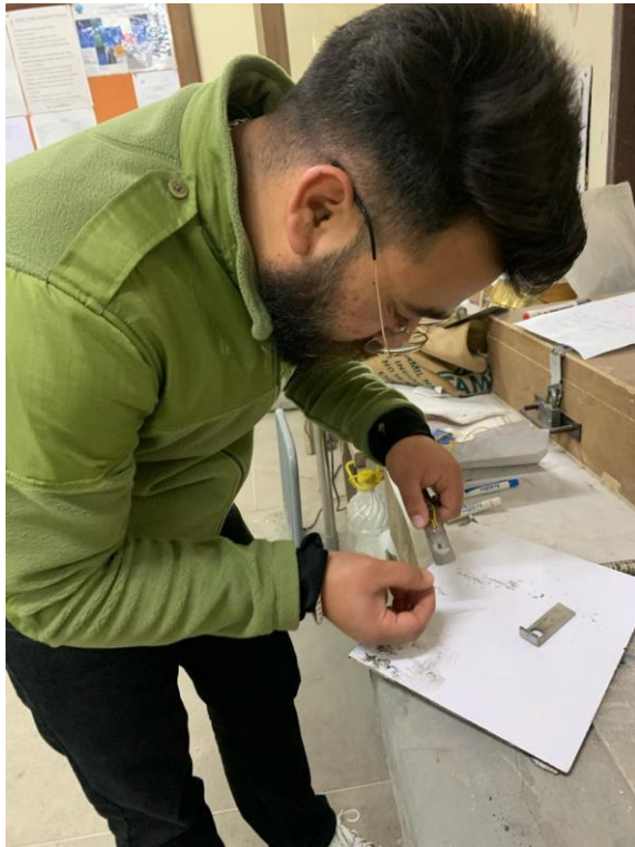
Fig.3.2 (a) Pasting strain gauges
