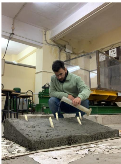
Fig.3.8 (c) Curing of retaining wall
