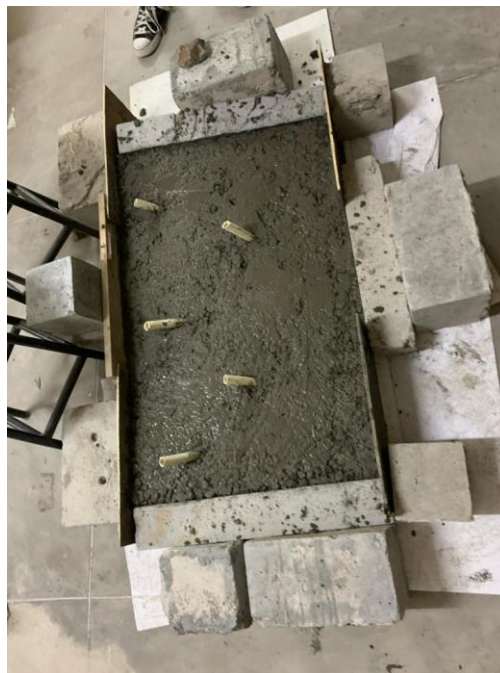
Fig.3.8 (b) Casting of retaining wall
