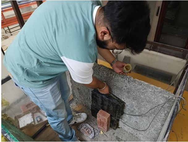
Fig. 3.13 (a) Strain gauges placement
