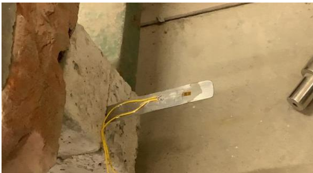
Fig. 3.2 (c) Calibrating strain gauges
