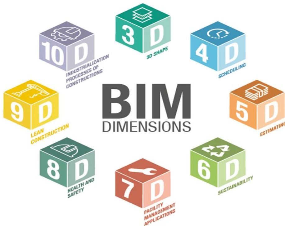
Figure 1.4: Dimensions of a BIM Project
