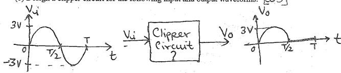
(c) Explain the working of the circuit given below and sketch the output  $(V_0)$  waveform.
