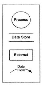
A data flow diagram (DFD) is a graphical representation of the "flow" of data through an information system. A data flow diagram can also be used for the visualization of data processing (structured design). It is common practice for a designer to draw a context-level DFD first which shows the interaction between the system and outside entities. This context-level DFD is then "exploded" to show more detail of the system being modeled.
