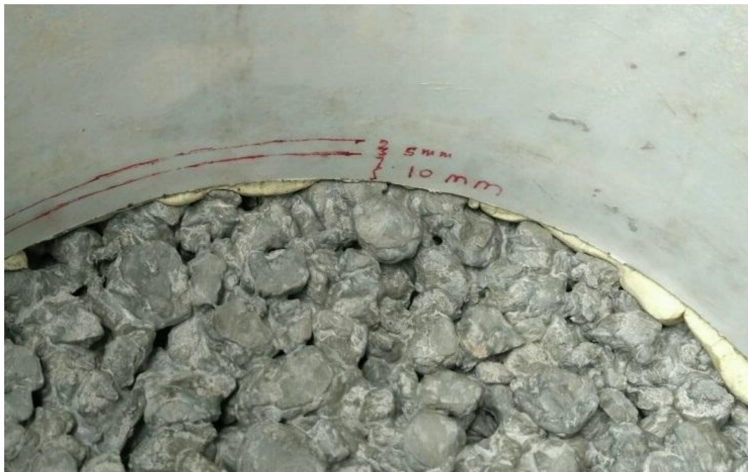
Fig. 4.9 Infiltration Ring Markings
