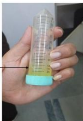
Fig. 11 Test for checking the solubility of the hydrogel
