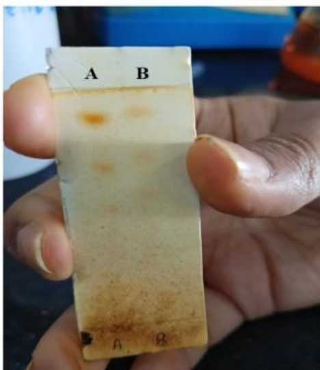
Fig. 9 TLC of curcumin sample; A = Standard sample of curcumin, B = Test sample of curcumin
