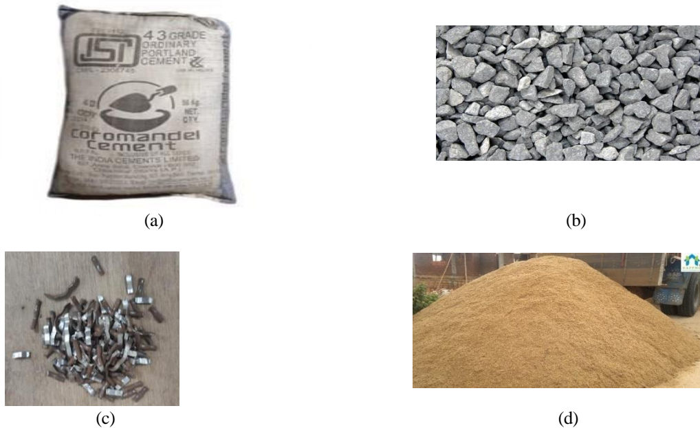
Fig. 3.1 (a) Portland Pozzolana Cement (PPC) (b) Coarse Aggregates (c) Steel Scrap fibers (d) Fine Aggregates
