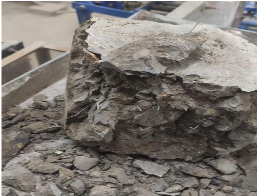
Fig 4.2 Picture of cube after testing
