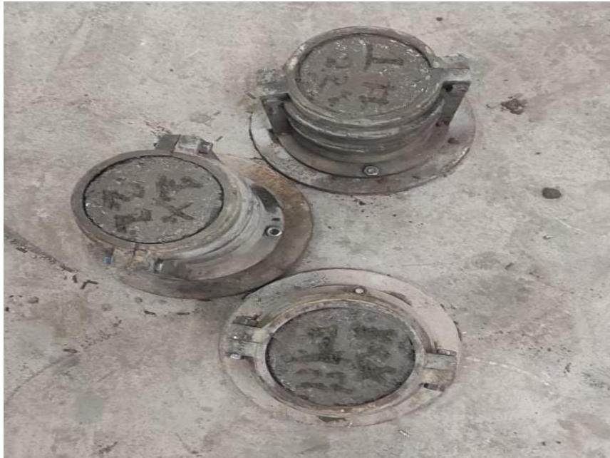
Fig 4.5 Casting of Cylinders
