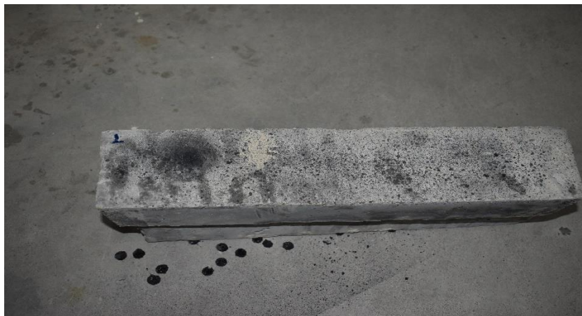
Fig 4.4 Speckle pattern on sample 1(RCC beam)
