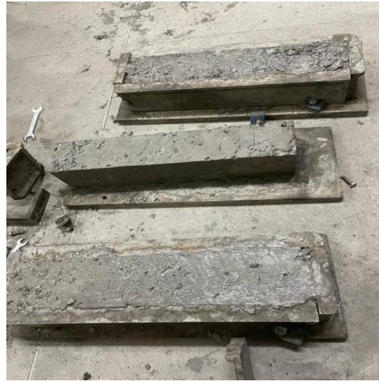
Fig 4.3 Beam before curing
