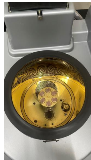
Fig 14(a): Stubs after gold plating.
