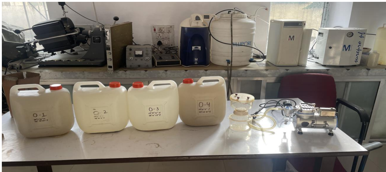
Fig 10: Collected sample along with a Vacuum pump
