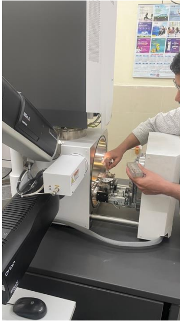
Fig 15(a): Stubs being placed in the SEM.
