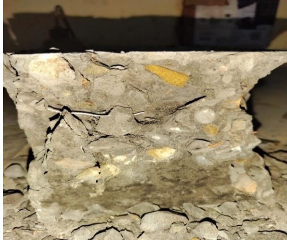
Fig 4.7 Placement of fiber after failure of cube
