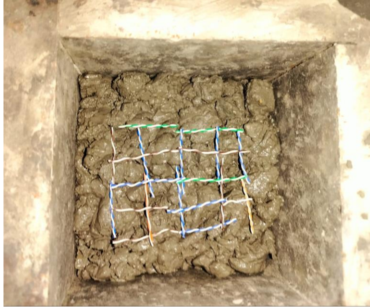
Fig. 4.11 Placement of double layered of fiber in Concrete Mix
