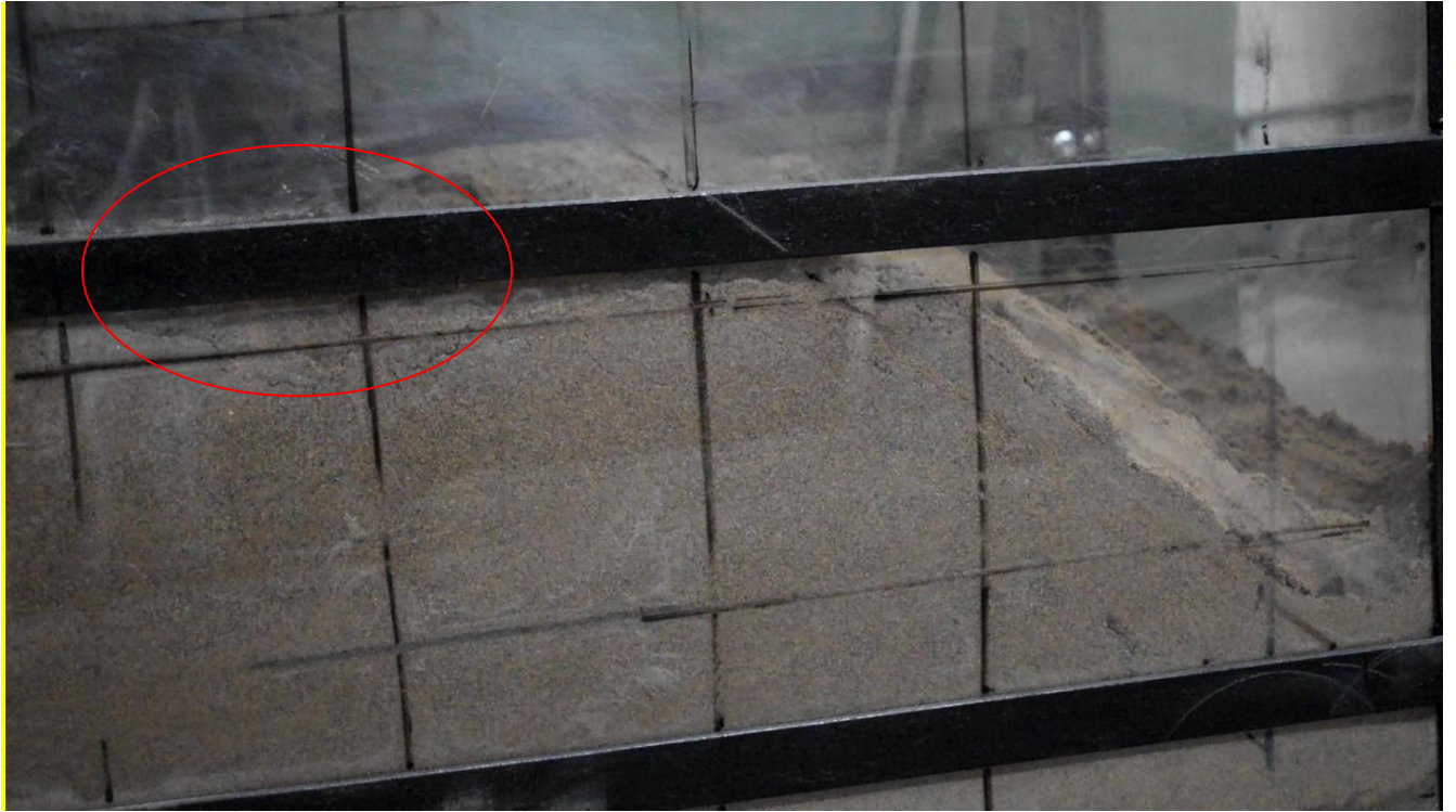
Figure 4.6 Shift of slope crest after applying the load
