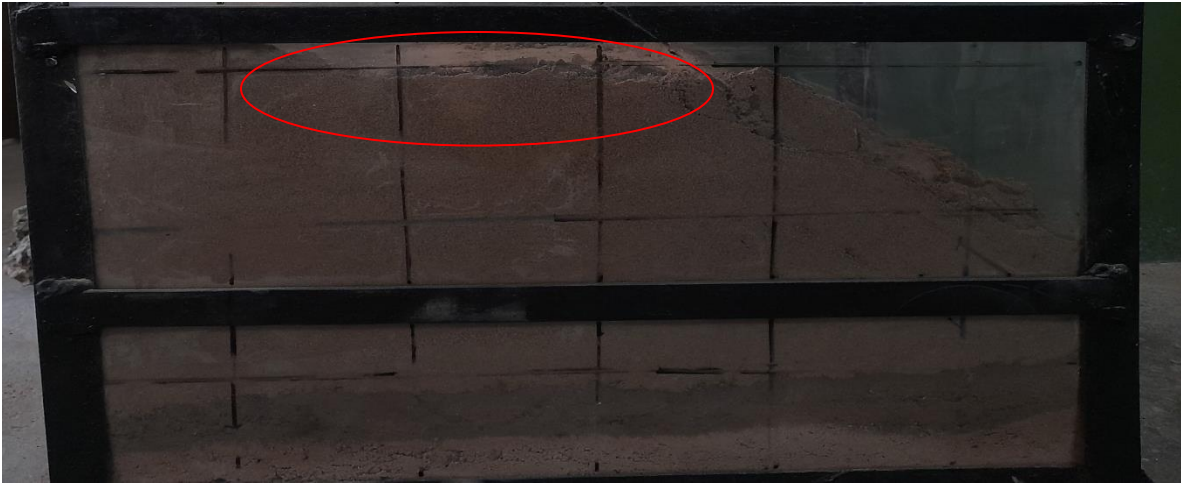
Figure 5.2 Sand slope after failure
