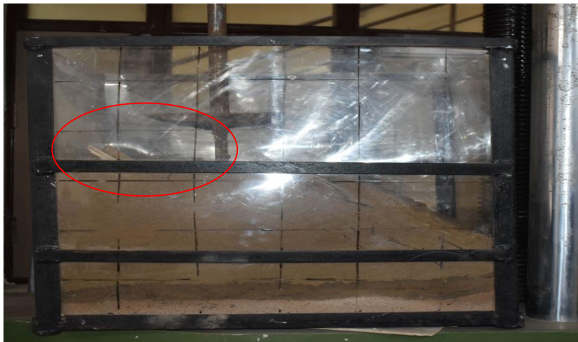
Figure 4.5 Load applied on the crest of the sand slope
