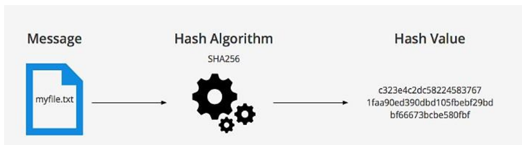
Figure 3.22: How hashing works in our project
