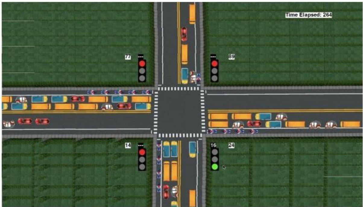
Fig 7 : Simulation showing green time of signal for vehicles moving left set to 24 seconds according to the vehicles in that direction
