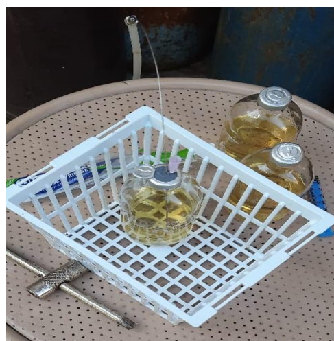
Fig. 4.4 Purging of N 2 in serum bottle containing Nutrient Broth
