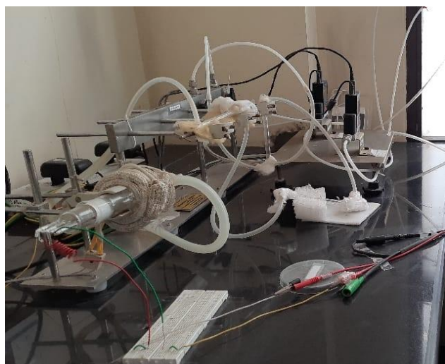
Fig. 4.26 Keithley's Picometer & Voltage Source Hydrogen Gas Sensor Setup
