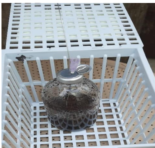
Fig. 4.3 Purging of N 2 in serum bottle containing Bushnell Haas broth
