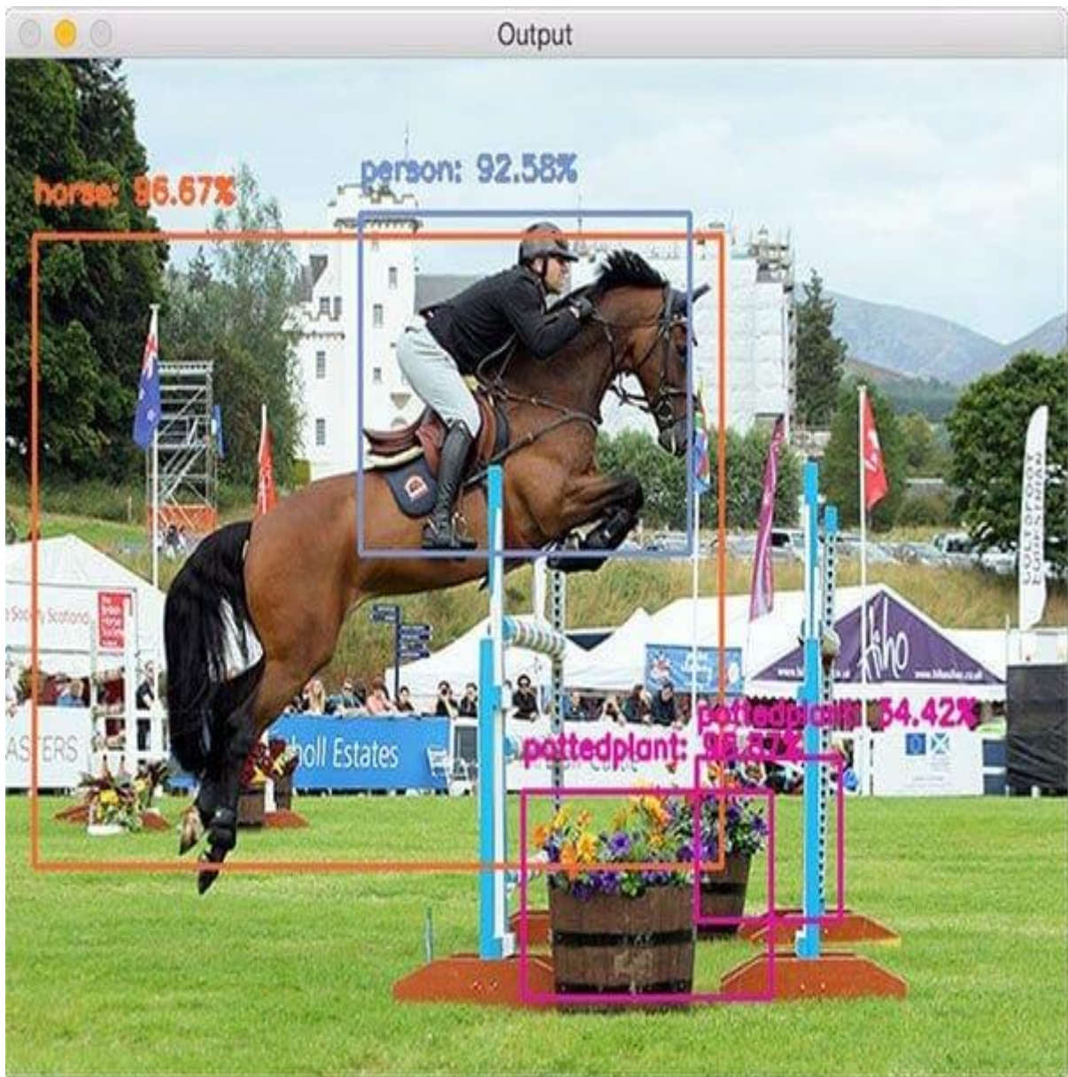
Figure1.2: Deep learning-based object detection detecting a person riding a horse and two potted plants. [3]
