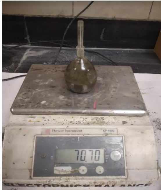
Fig. 4.6 Specific gravity of cement
