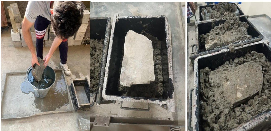
Fig.4.11 Casting of stone concrete block
