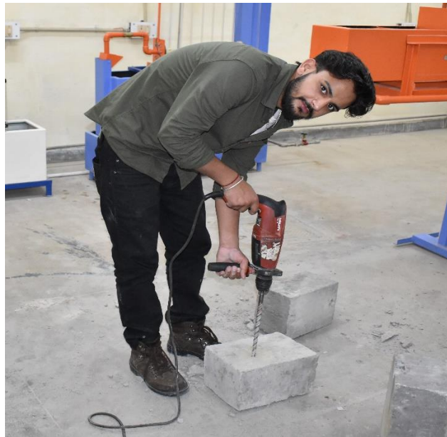
Fig. 4.13 Drilling holes in blocks
