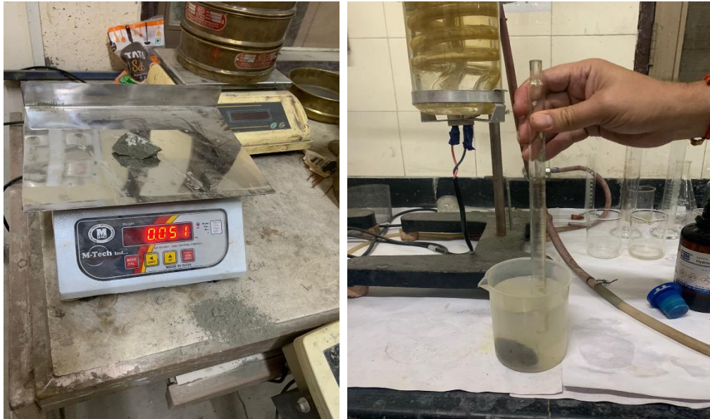
Fig. 5.1 Acid test on stone
