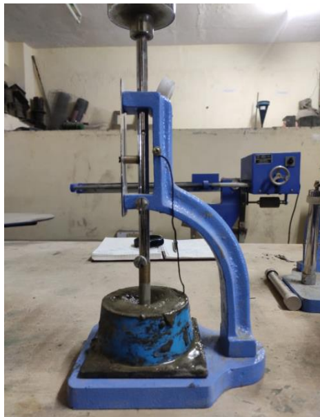
Fig 4.5 Normal consistency with vicat's plunger
