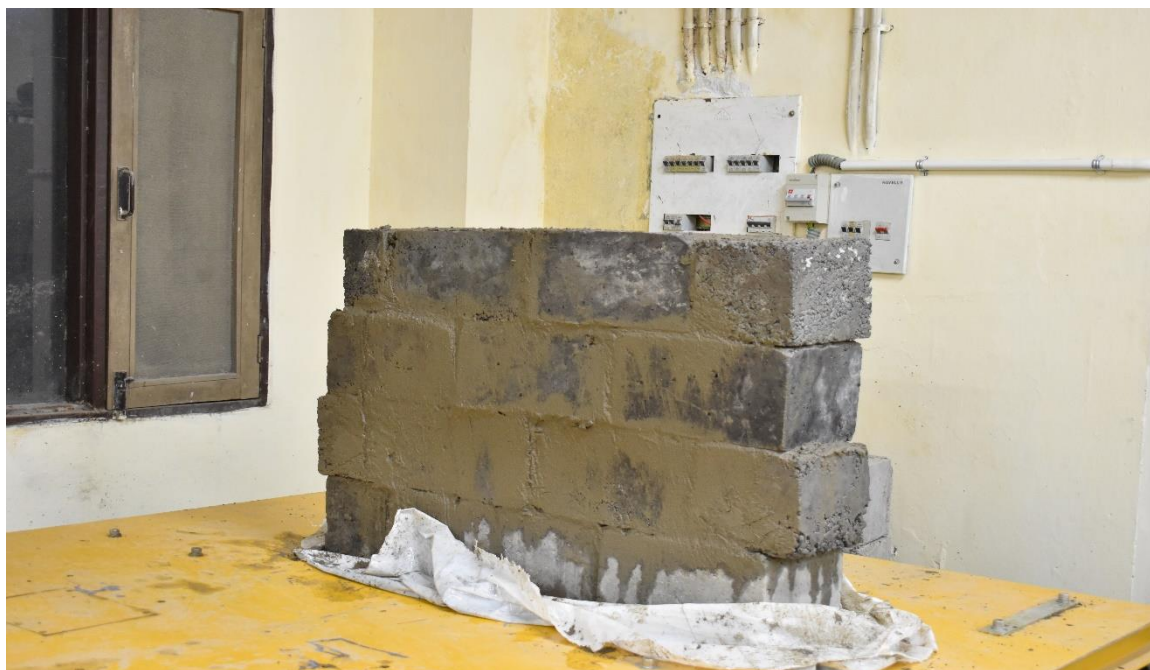
Fig. 4.14 Stone concrete block wall
