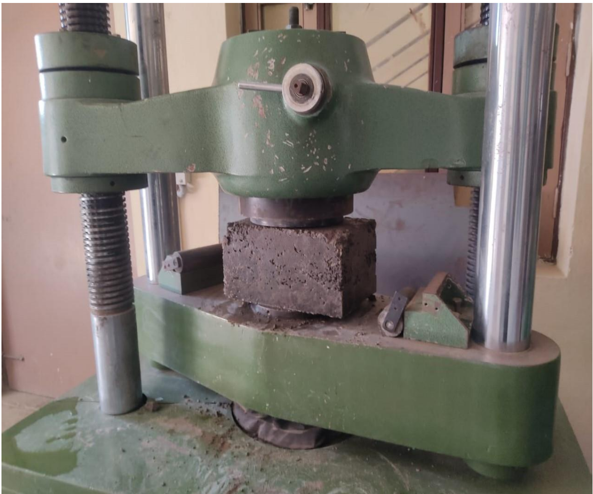
Fig. 5.3 Testing of blocks in UTM
