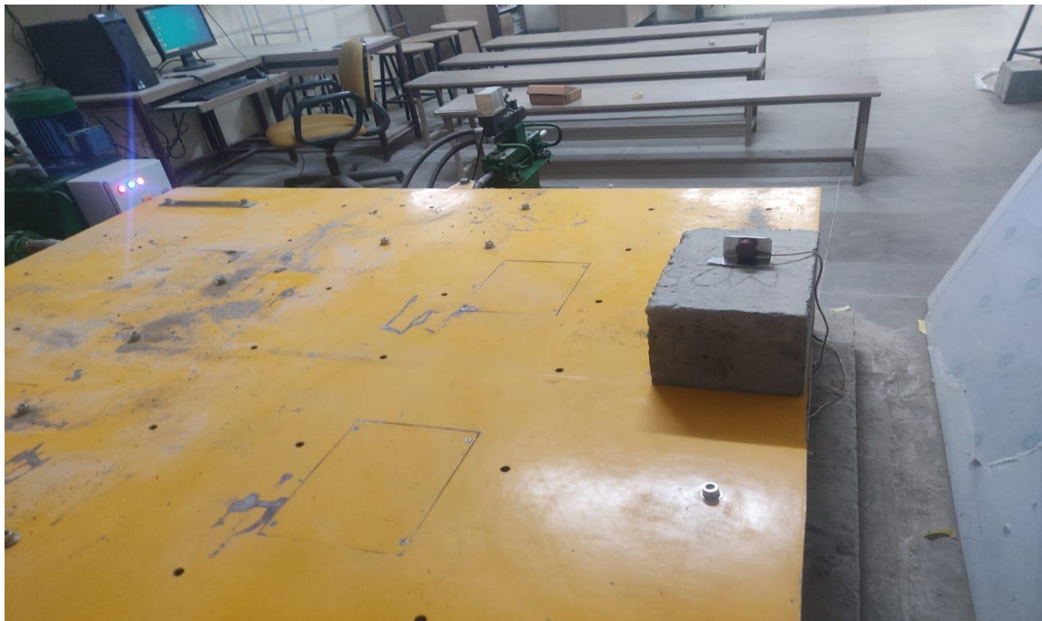
Fig. 5.5 Sine sweep test on block
