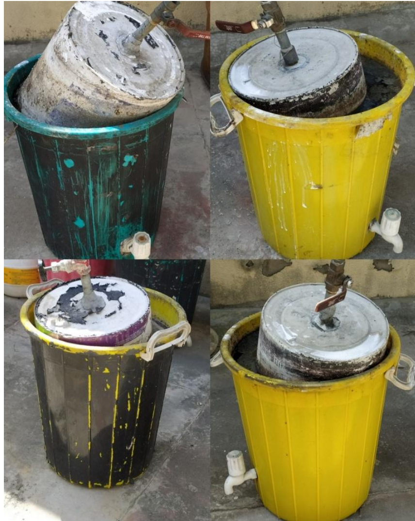
Figure 3.1) Anaerobic digesters used for biogas production.
