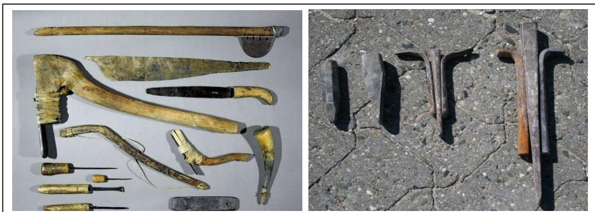
Figure 1.7 Ancient tools and plug and feather toolset
