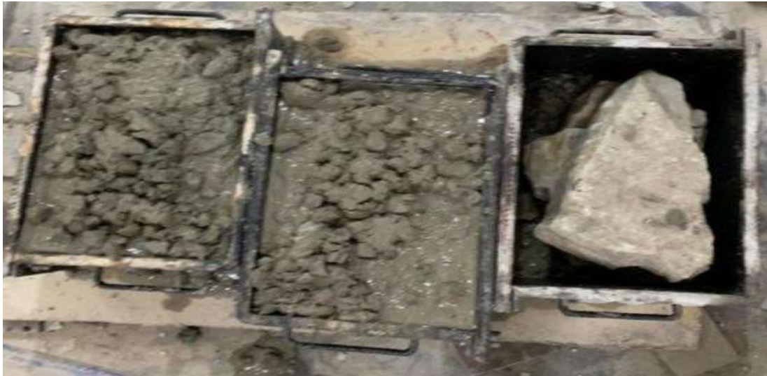
Figure 3.12 Casting of blocks
