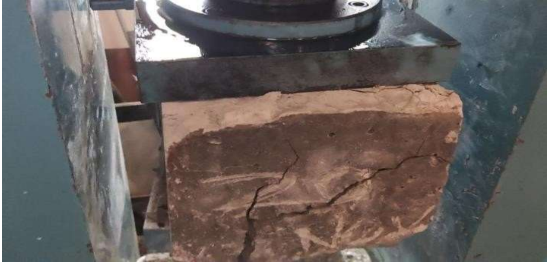
Figure 3.16 Cube after application of load
