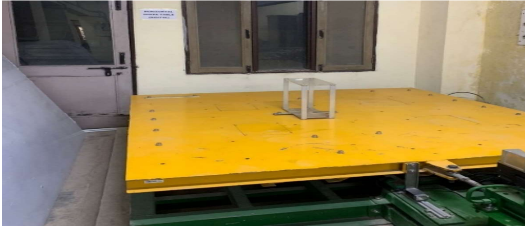
Fig 3.17 Uniaxial shake table
