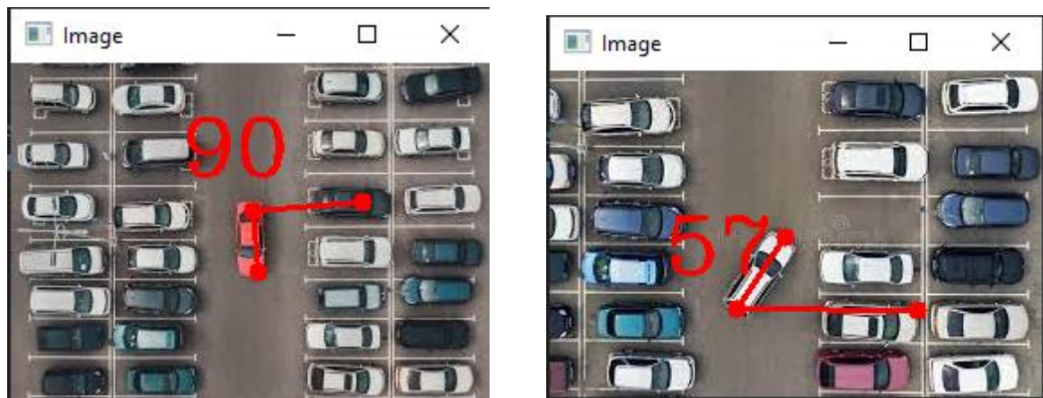
Fig. 4.4 Angle calculation for classifying wrongly parked vehicles
