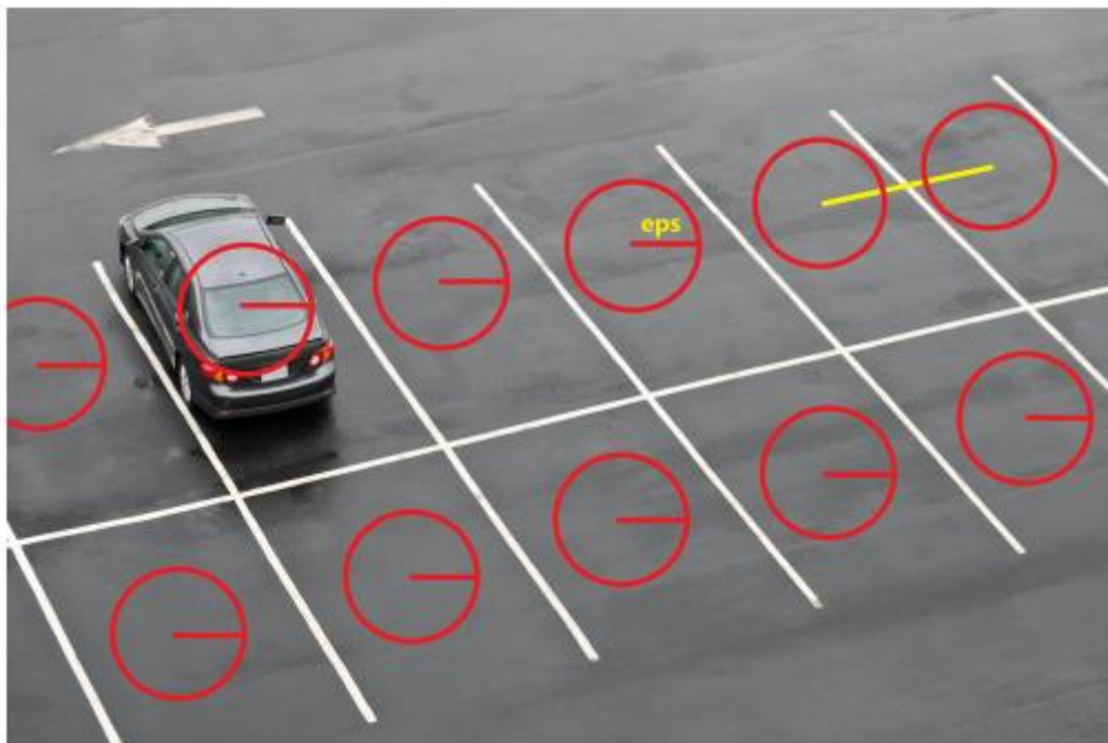
Fig. 4.3 Detecting the vacant spaces
