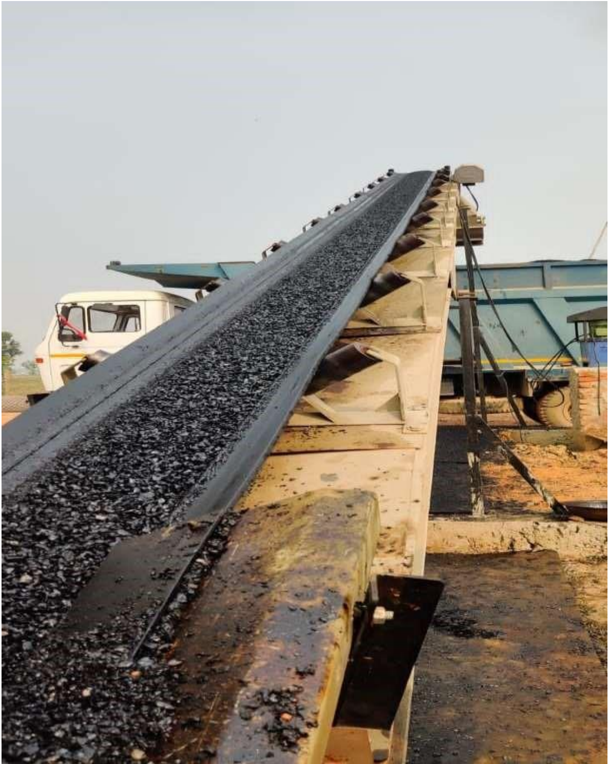
Figure 3.2: Dispatching of bitumen from bitumen plant
